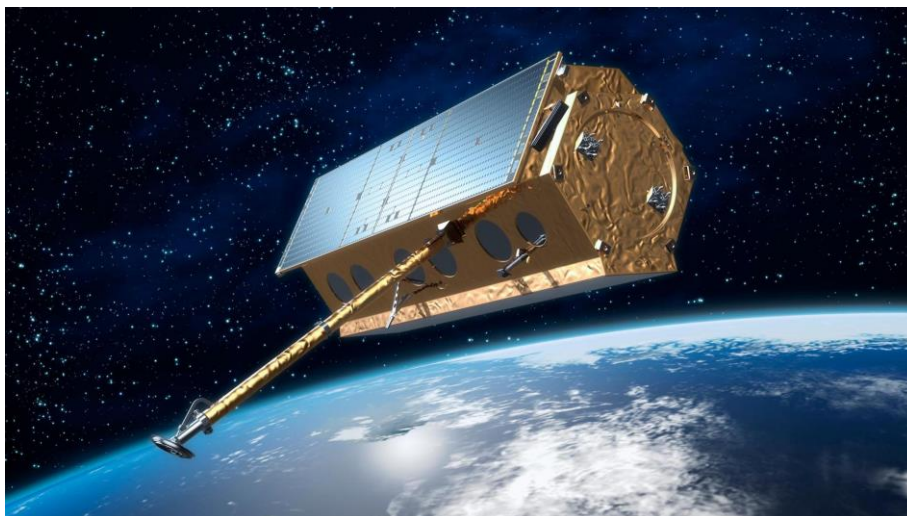
Figure 9: Computer image of TerraSAR-X satellite with X-band radar antenna (bottom left) (Source of image: German Aerospace Center ( www.dlr.de ))
