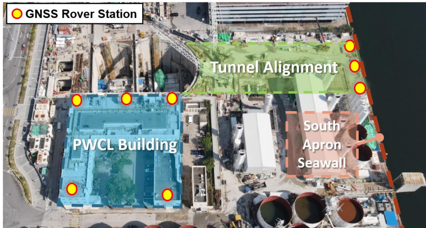
Figure 2: Phase 1 GNSS monitoring: at rooftop of PWCL Building (left) and along South Apron seawall (top right)
