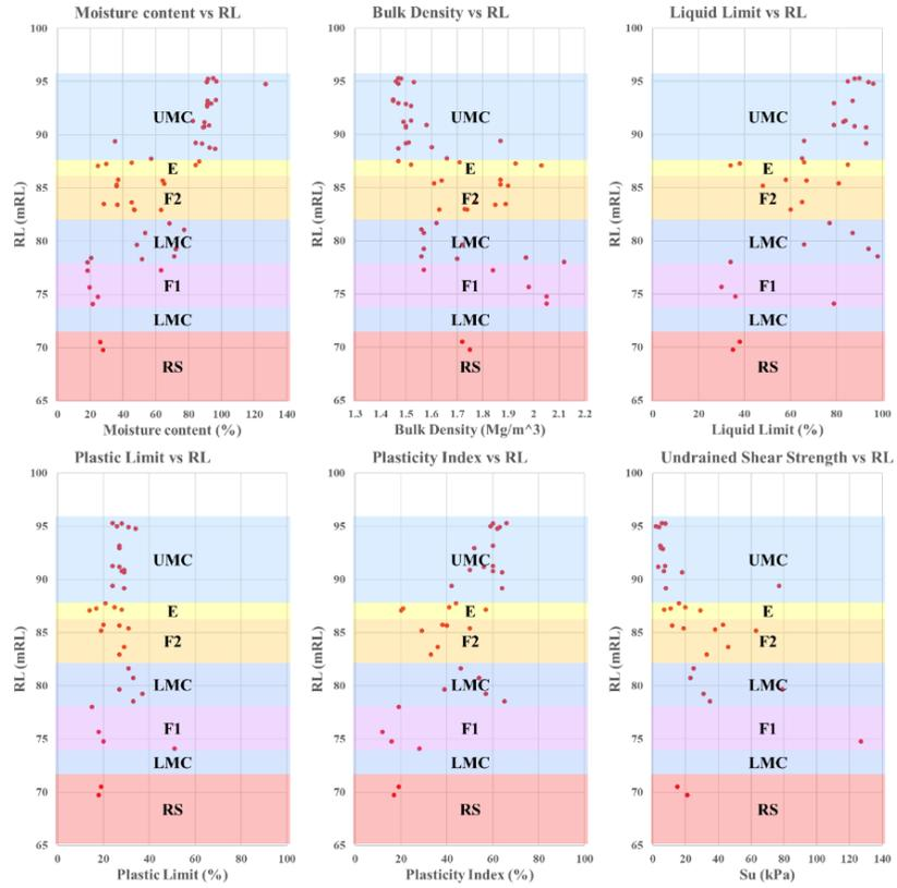
Figure 4 Geotechnical parameters from the nearest boreholes to the DSM trial panel.
