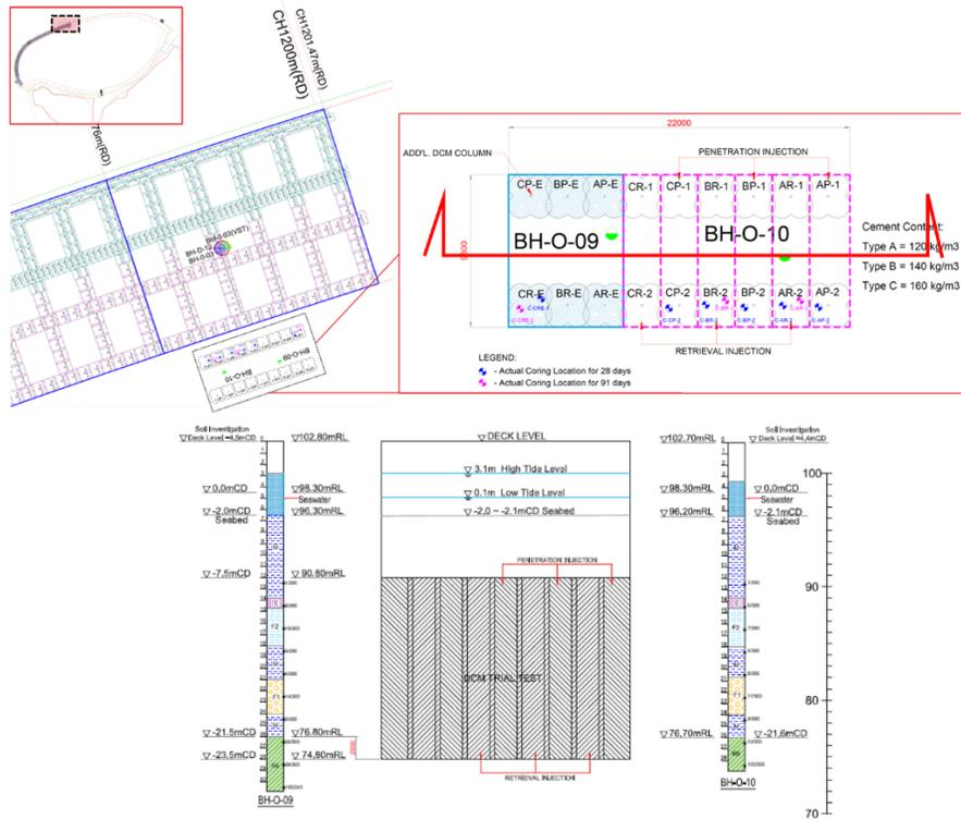
Figure 5 Location of the Trial DSM Panel, constructed adjacent to the working DSM walls.
