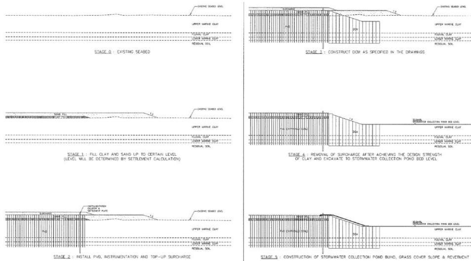
Figure 2 Construction sequence of the polder, taken near Section S1. The formation of the dike at the edge of reclaimed land is not shown here.
