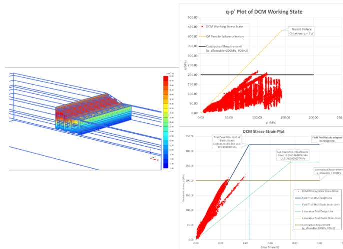
Figure 18 Assessment of DCM internal stress under service loads.
