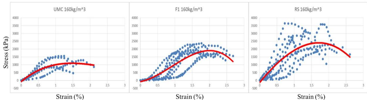
Figure 11 DSM Laboratory trial test results for the same cement content across various soil types.
