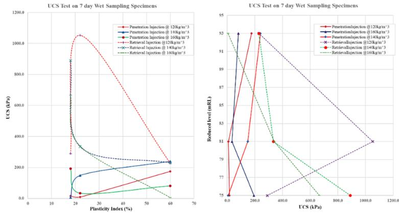
Figure 13 Wet sampling specimen, left: UCS vs PI, right: UCS variation over depth.
