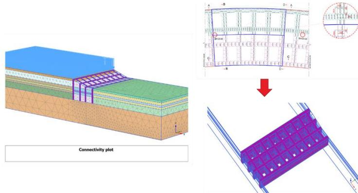
Figure 17 3D numerical analysis of the DSM cell block
