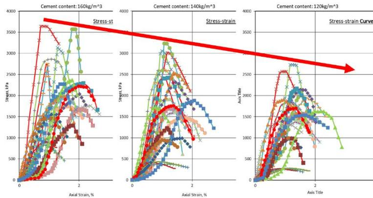
Figure 9 Aggregated laboratory DSM trial mix results for all soil types, separated by cement content.
