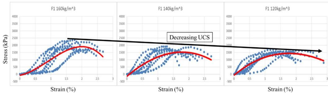
Figure 10 DSM Laboratory trial test results for F1 soil type, across various cement contents.
