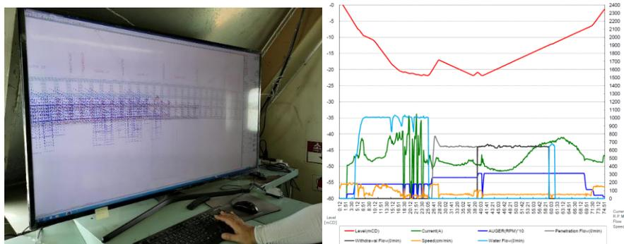
Figure 8 Acquisition of data as seen on board the DSM Barge. Left: DSM As-Built Positions. Right: Mixing parameters such as cement flow rate, water flow rate, auger position, auger rotation speed, etc.
